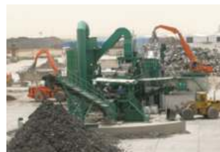
SMG shredding system converting bulk scrap metal into uniform fragments optimized for EAF steelmaking.
